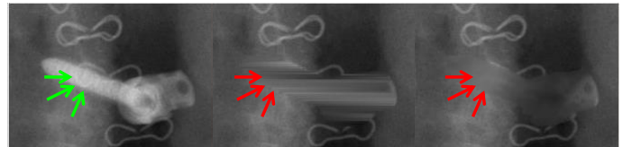
Fig. 1. High contrast structure clearly visible in metal shadow of screw (green arrows, left), linear 1D interpolated projection (middle), linear 2D (right). The interpolation erases the structures in the metal shadow.
